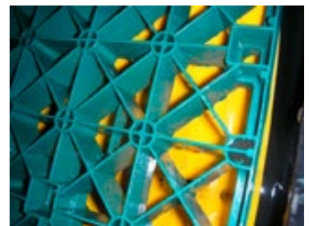
Cleaned, residue-free system; the area of the flow separator is displayed here
