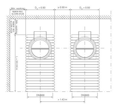
The above sections of the installation manual describe the standard installation as individual system. The following describes the recommendations for the arrangement of multiple systems and the required minimum distances.
